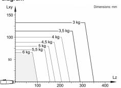
The KR 6 R900 CR is designed for a rated payload of 3 kg in order to optimize the dynamic performance of the robot. With reduced load center distances, higher loads up to the maximum payload may be used. The specific load case must be verified using KUKA.Load. For further consultation, please contact KUKA Support.
