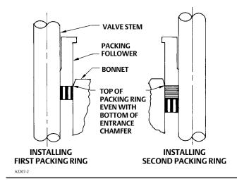
For graphite packing, tighten the packing flange nuts to the maximum recommended torque shown in table 7. Then, loosen the packing flange nuts, and retighten them to the recommended minimum torque shown in table 7.
