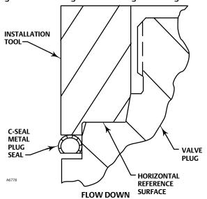
NOTE: PRESS THE INSTALLATION TOOL OVER THE VALVE PLUG UNTIL THE TOOL CONTACTS THE HORIZONTAL REFERENCE SURFACE OF THE VALVE PLUG.
