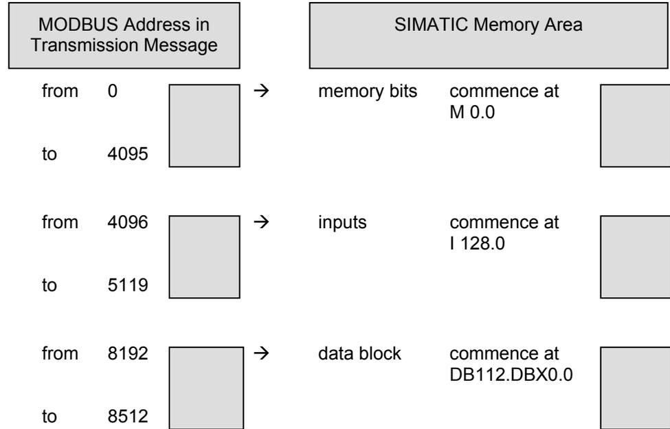
The Modbus addresses from 0 to 4095 access the SIMATIC memory bits commencing at memory bit M 0.0; i.e. length of area = 4096 bits = 512 bytes, which means last memory bit = M 511.7.
