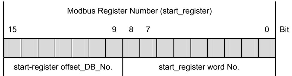
For further address generation, the driver uses the “Base DB number” (commence at DB yyyyy) entered in the dialog box “**Conversion of Modbus Addressing for FC 04.**”
