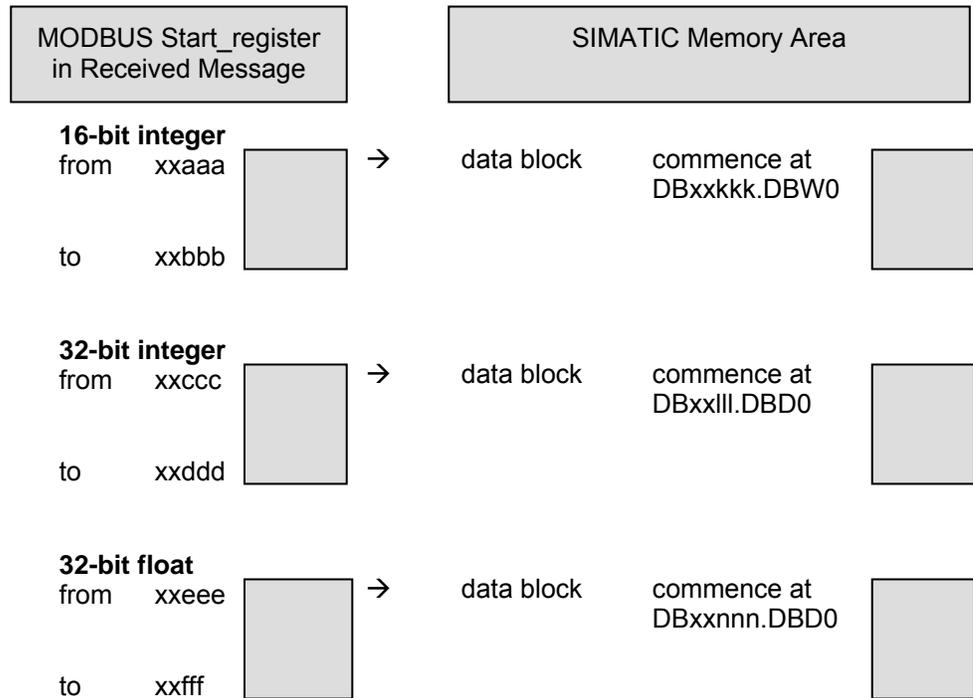
The DBs which are normally organized in bytes are in this instance interpreted by the driver as follows.
