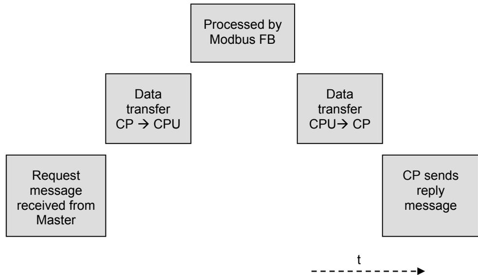
The reaction times depend on the cycle time of the CPU program (Modbus FB) and the CPU type (data transfer CPU↔CP).
