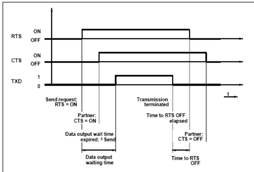
Figure 7-1 Time Diagram for Automatic Use of the RS 232C Secondary Signals
