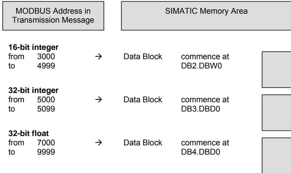
You can use Modbus register address 3000 to access data block 2 commencing at DBW 0 in the SIMATIC system.; i.e. length of area = 2000 words, which means last data word = DB2.DBW3998 (last accessed byte is DB2.DBB3999).
