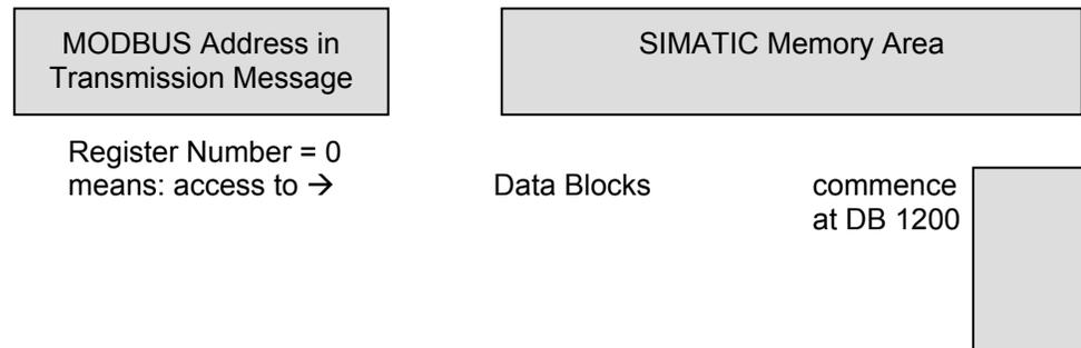
You can use Modbus register address 0 to access data block 1200 commencing at DBW 0 in the SIMATIC system. Higher Modbus register addresses  $\geq 512$ , 1024, etc.) access the following DBs DB 1201, 1202, etc.
